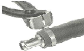
Grip the outer edge of ear firmly and cut through it with either pincers.
