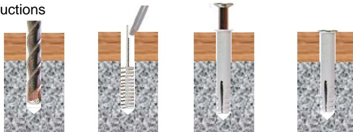
1. Drill correct diameter hole through fixture to correct depth in base material.
