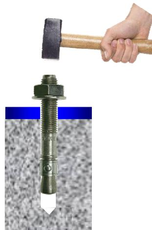
Insert assembled anchor through fixture into concrete
