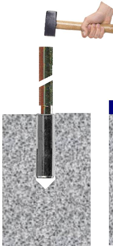
Insert anchor into concrete and hammer wedge home using correct setting punch
