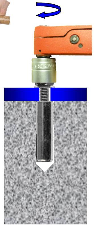
Tighten with torque wrench to recommended torque
