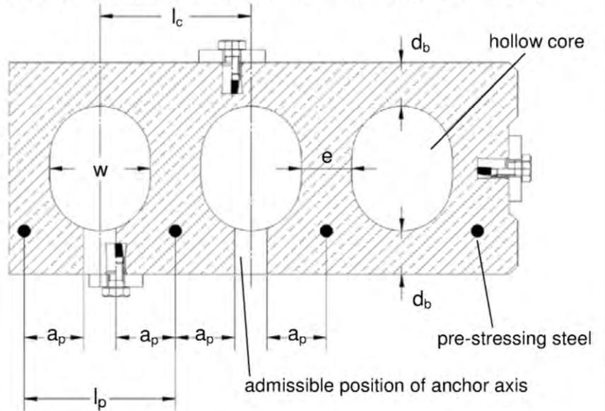
**Minimum spacing and edge distance of anchors and distance between anchor groups in precast pre-stressed hollow core slabs**
