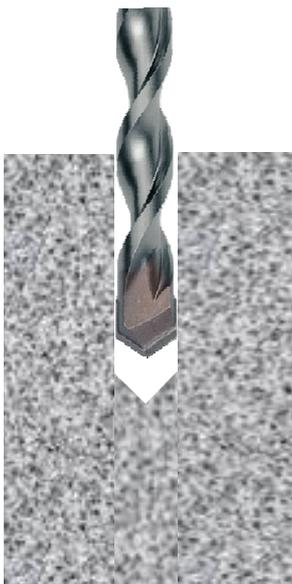
Drill correct diameter hole to correct depth
