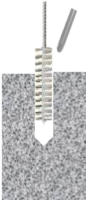
Clean hole by brushing and blowing to remove all dust and drilling debris
